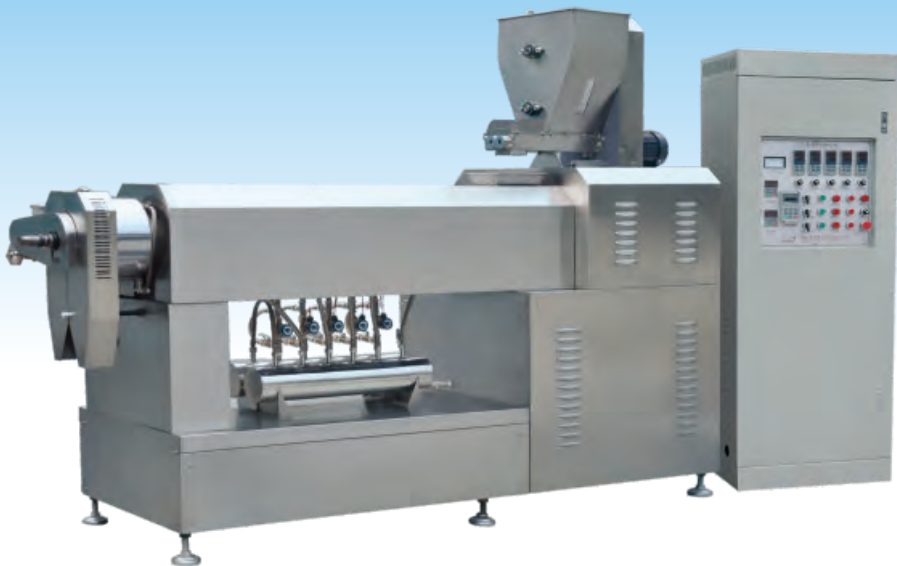
ZH2000-100 Single-screw Extruder
